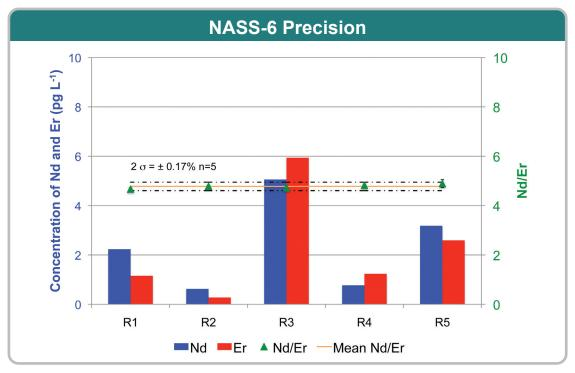
**Figure 9.** The interpretation of dissolved REEs requires high quality concentration values from which very precise patterns and elemental ratios can be determined. Three NASS-6 replicates, run on five different analytical dates, indicate good precision for concentration data and better than ± 3.5% (2-sigma) for LREE/HREE (Nd/Er) ratios.
