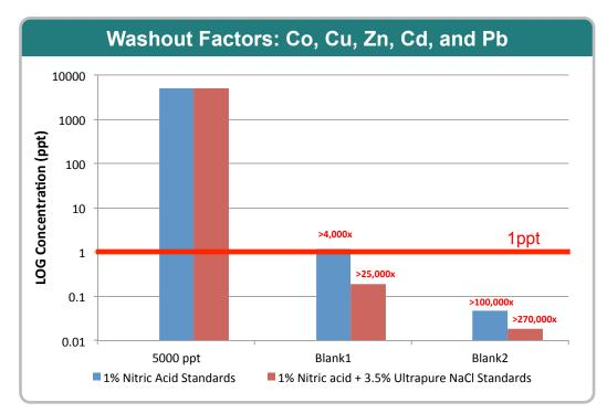
**Figure 26.** Washout in Preconcentration mode is excellent with both 1% nitric acid calibration standards and matrix-matched standards. Matrix matching the standards with seaBlank is not required for Preconcentration mode, but it enhances washout.
