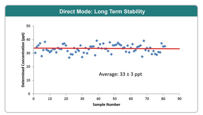
**Figure 36.** Long term stability of Cr in synthetic seawater shows >14 hours of repeated determinations with internal standard correction. Direct mode automatically diluted the sample inline by 10x. The determined concentration in the synthetic seawater was  $33 \pm 3$  ppt.
