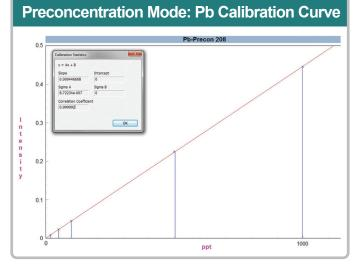
**Figure 32.** Autocalibration from a single 1000 ppt calibration standard. Calibration curve was matrix matched to ~3% TDS.
