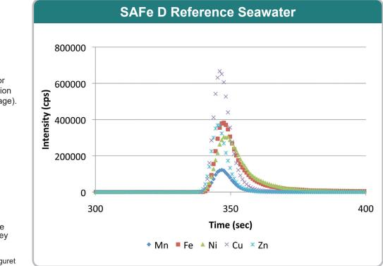
**Figure 14.** Elution profiles for a selection of first row transition metals (2 point running average).
