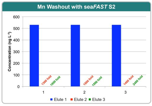
**Figure 12.** Three replicates of a three step elution are plotted. The first step, after loading NASS-6, recovers trace metals from the column. Two subsequent elution steps illustrate greater than a 1000-fold washout, indicating minimal sample to sample carryover. Low carryover is sufficient to measure trace metals in a wide variety of oceanic environments.
