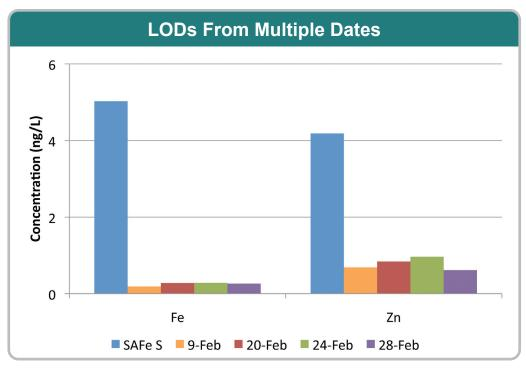
**Figure 15.** Limits of detection for contamination-prone elements (Fe and Zn) are in the high pg L<sup>-1</sup> range and are reproducible on a day-to-day basis. These limits of detection are appropriate for determination of ultra-trace metal concentrations in open ocean surface seawater.
