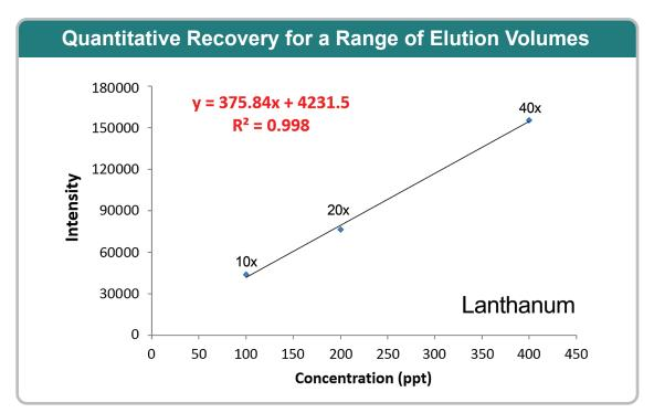
**Figure 6.** By adjusting elution volume (1000, 500, to 250  $\mu$ L), 10 mLs of Indian Ocean surface water (with 10 ppt REE spike) is concentrated 10, 20, and 40x. A linear correlation between concentration and intensity indicates that even 250  $\mu$ Ls is sufficient for quantitative recovery.
