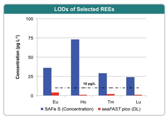
**Figure 8.** Limits of detection are compared to SAFe surface water concentrations. Matrix removal combined with a 20-fold preconcentration factor is sufficient to determine the lowest level of REEs in open ocean seawater.
