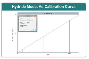
**Figure 34.** Autocalibration from a single 1000 ppt calibration standard. Calibration curve was matrix matched to ~3% TDS.
