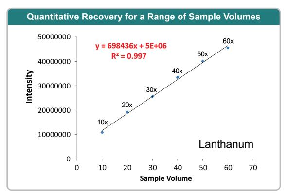
**Figure 7.** By adjusting sample volume (10 - 60 mL), Indian Ocean surface water (with 10 ppt REE spike) eluted in 1 mL is concentrated 10 - 60x. A linear correlation between concentration and intensity indicates the columns capacity to process large volume samples with quantitative recovery.
