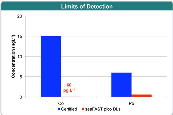
**Figure 13.** Limits of detection are compared to NASS-6 certified values. Matrix removal combined with a 20-fold preconcentration factor is appropriate for many seawater applications. If lower detection limits are required, the system can easily be programmed for larger preconcentration factors.
