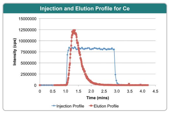
**Figure 5.** A comparison of a sea*FAST* S2 inline elution profile with a sea*FAST* S2 offline injection is shown above. Offline fraction collection of programmable elution volume is injected to the ICPMS with a micro*FAST* system. A profile collected from a sample eluted in 200  $\mu$ L and introduced at 100  $\mu$ L min<sup>-1</sup> illustrates two minutes of steady state signal.
