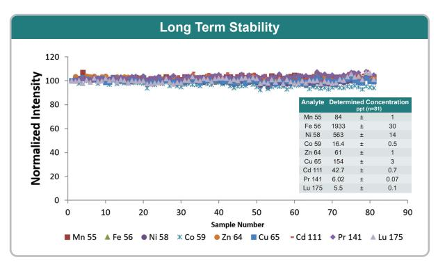
**Figure 37.** Common transition metals and selected rare earth elements (REEs) were determined in synthetic seawater consecutively for over 14 hours (n=81). Auto-matrix-matched blanks and QC standards are not shown, for clarity. Average precision over 14 hours was better than 2% with internal standard correction. REEs were spiked at 5 ppt.
