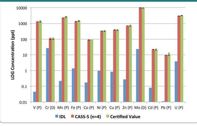
**Figure 25.** Results for NASS-6 and CASS-5 Seawater Reference Materials are shown. Elements determined with the sea*FAST* S2 are accurate and precise for elements with certified concentrations from < 10 ppt to > 10 ppb.
