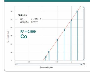
A sub-ppt standard addition calibration prepared by auto-spiking a DI water sample, background subtracted.
