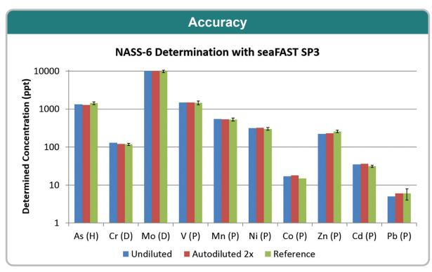
**Figure 38.** NASS-6 was analyzed in all three modes, Preconcentration (P), Direct with fixed 10x inline dilution (D) and Hydride (H). NASS-6 was run undiluted and with a 2x autodilution using automatic, inline matrix matching with seaBlank ultrapure sodium chloride solution. The sea*FAST* achieves excellent accuracy in all three modes, with and without autodilution.
