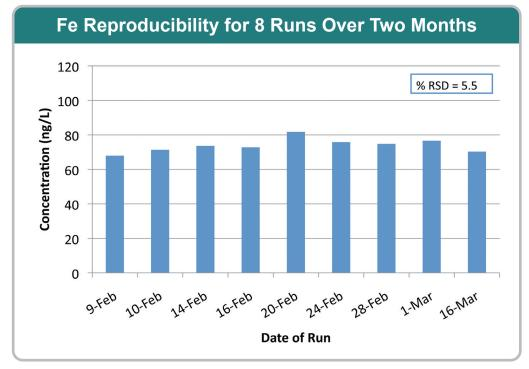
**Figure 16.** An internal laboratory standard of Ross seawater collected from the Southern Ocean is run several times on each of 9 discrete analytical dates. Excellent day-to-day reproducibility is illustrated for Fe, a difficult contamination-prone element.
