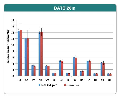
**Figure 3.** Single digit picomolar (<1 to 15 pM) concentrations of REEs are routinely determined in surface samples (20m) from the Bermuda Atlantic Timeseries Station (BATS). The error bars (2 SD) illustrate the precision of the method, whereas accuracy is demonstrated through agreement with consensus values. Data courtesy of Katharine Pahnke, Melanie Behrens and Ronja Paffrath, Max Planck Research Group for Marine Isotope Geochemistry.
