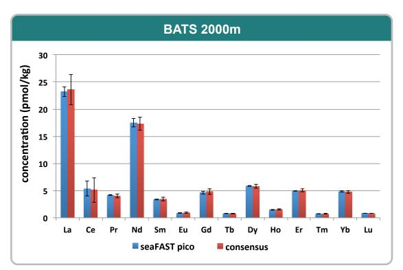
**Figure 4.** Similar to Figure 3, REEs determined and consensus concentrations for a deep sample (2000m) from the Bermuda Atlantic Time-series Station (BATS) are plotted. The error bars (2 SD) illustrate the precision of the method, whereas accuracy is demonstrated through agreement with consensus values. Data courtesy of Katharine Pahnke, Melanie Behrens and Ronja Paffrath, Max Planck Research Group for Marine Isotope Geochemistry.
