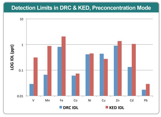
Figure 27. Detection limits are near or better than 1 ppt on a quadrupole ICPMS (n=10,  $3\sigma$ ).
