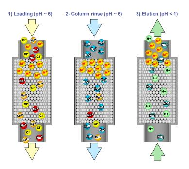
**Figure 1.** Image and schematic of the sea*FAST* preconcentration column. At a pH  $\sim$  6, transition row metals are chelated on the preconcentration column, while matrix elements (group 1 and 2) are flushed from the column.
